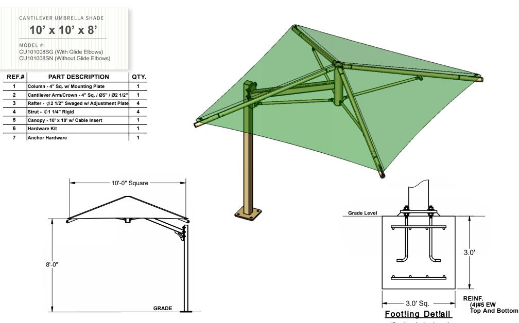
\*Footing design based on 1500 PSF soil bearing pressure.
