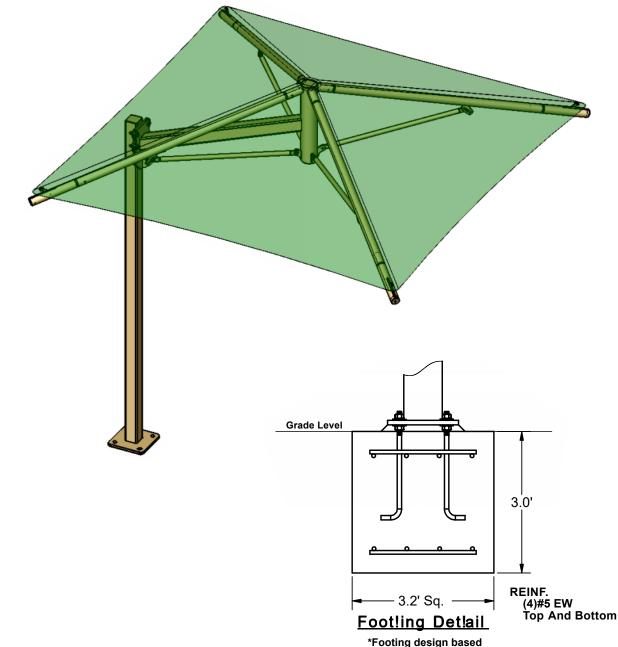
\*Footing design base on 1500 PSF soil bearing pressure.
