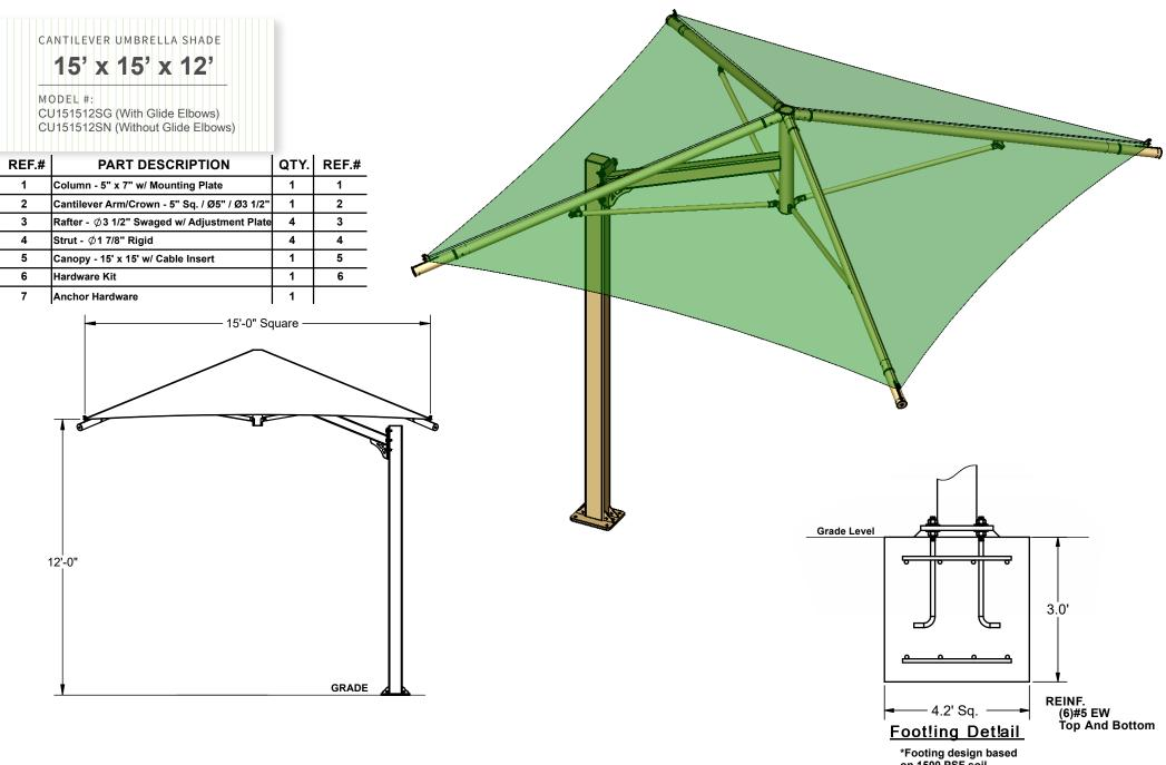
on 1500 PSF soil bearing pressure.
